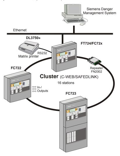
An optical Ethernet network (C-WEB/LAN) allows up to 14 clusters with up to 16 stations to be operated on one network. A maximum of 64 stations is supported in total.
